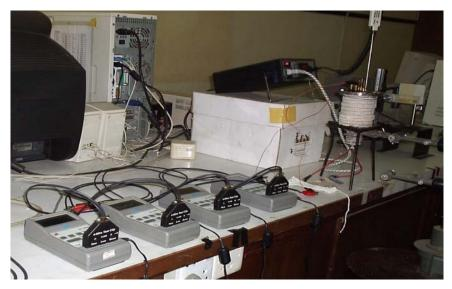
Figure 4 Photograph of the experimental setup for the measurement of DC conductivity
