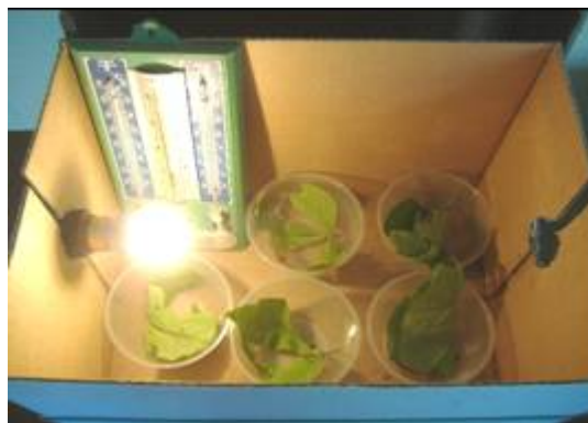
Figure 2. Temperature tolerance test conducted by insetting a 5-watt bulb for maintenance of 40°C
