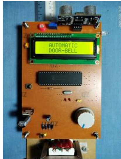
Figure 6. The title display illuminate on initial power up condition
