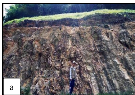
Fig 9. (a) Highly weathered of banded quartzite at near Kadaik Dam (Loc. N16°44'30.1" E 97°28'1.5" Facing 72°) (b) Quartzite with poorly jointed nature at near Kadaik Dam (Loc. N16°44'34.1" E 97°27'59.5" Facing 102°)
