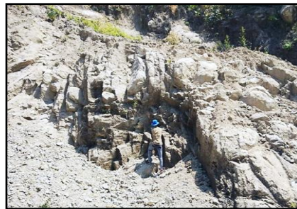
Fig 7. Vertical jointed nature of gneiss at near Palat Village (Loc.N16°41'12.7"E97°25'55.6", Facing174°)
