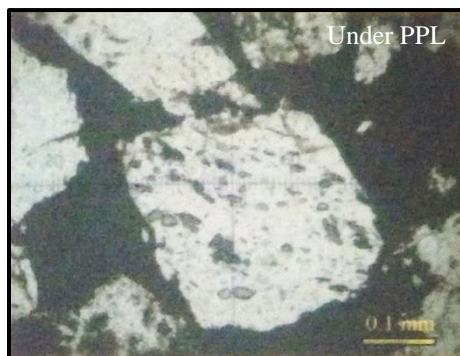
Fig.12 Mineral inclusions in quartz grain from upper Irrawaddy Formation
