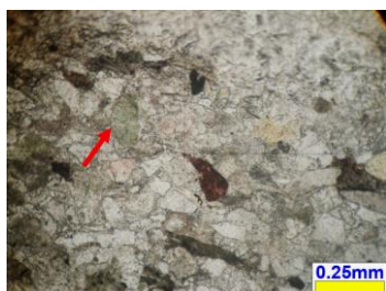
Figure 10. Photomicrograph showing authigenic chlorite mineral altered from feldspar (arrow) (under PPL) (Loc.821999).
