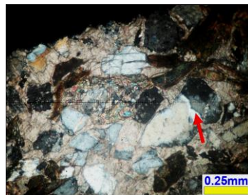
Figure 8. Photomicrograph showing quartz overgrowth (silica cementation) nature (arrow) (between X.N) (Loc. 836999).
