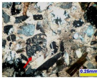
Figure 11. Photomicrograph showing the detrital grains are dissolution by calcite (arrow) (between X.N) (Loc. 833998).
