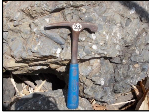
Figure (10) Massive, poorly sorted rock materials cemented by calcareous sandy matrix in Paunggyi Formation. (Loc. N17° 41' 06.8", E94° 58' 26.5", Facing; 70°)
