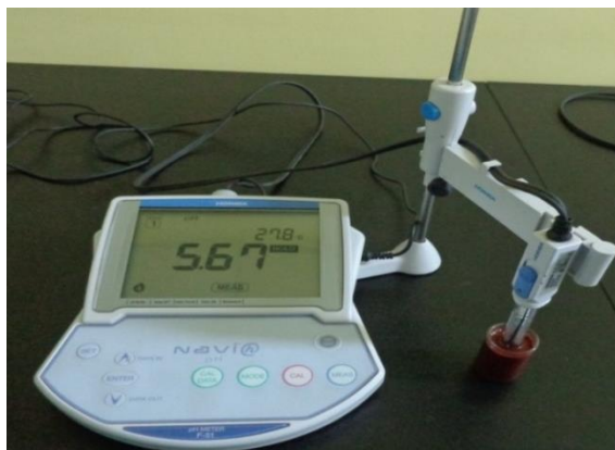
Figure (7) Measuring pH for teak leaves dye solution with pH meter.
