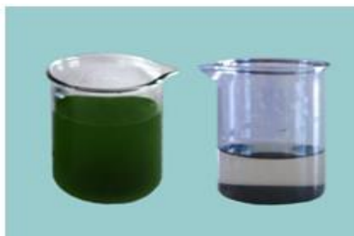
Figure (10) Photograph of catalytic degradation of residual dye in wastewater by using Mn 2 O 3 nanoparticles
