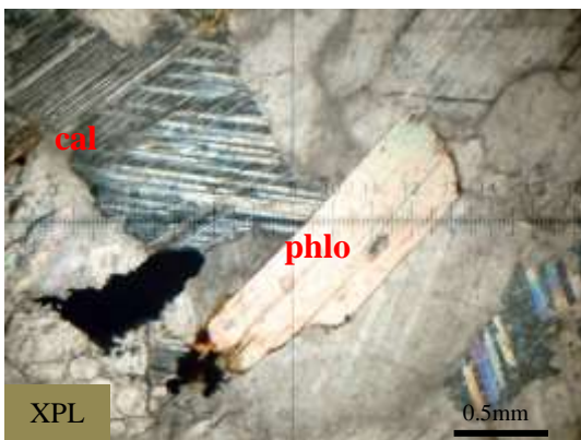
Fig. (19) Foliation direction with the alignment of calcite crystal and phlogopite crystal in phlogopite marble (XPL)
