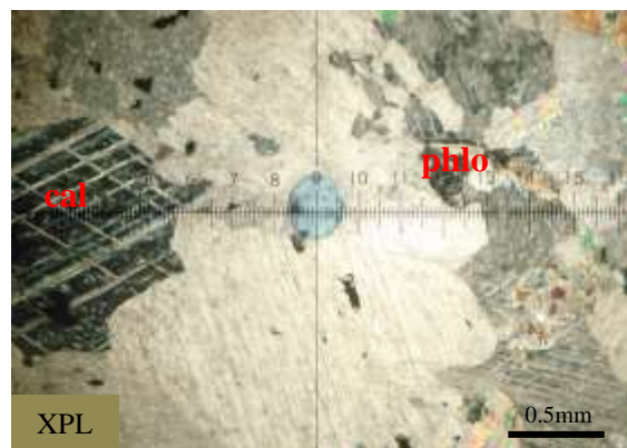
Fig. (20) Rhombohedral cleavage of calcite cleavages in phlogopite marble (XPL)
