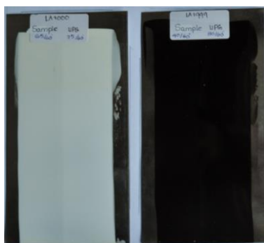
Figure (1) Comparison of weathering test (Prepared Paint and Standard UPG Paint).
