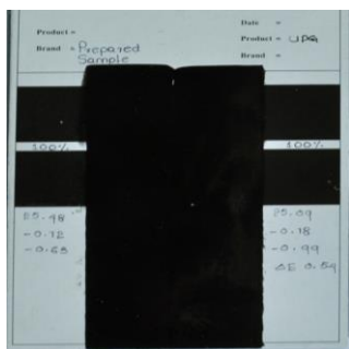
Figure (3) Comparison of hiding power test (Prepared Black Paint and Standard UPG Black Paint).
