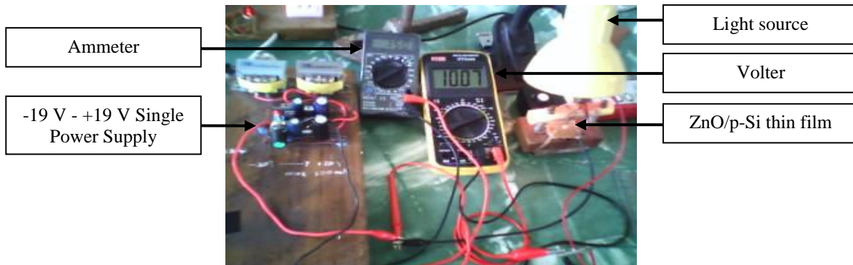
Fig. 2 Experimental setup of I-V characteristic measurement
