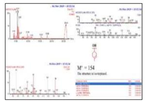
Figure (4.f) GC-MS spectrum of compound 6 from essential oil at RT 6.260 min
