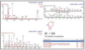
Figure (4.1) GC-MS spectrum of compound12 from essential oil at RT 9.163 min
