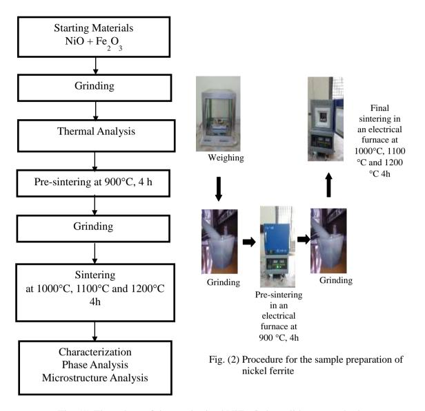
Fig. (1) Flow chart of the synthesized NiFe<sub>2</sub>O<sub>4</sub> by solid state method
